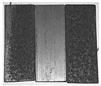
Figure 10: Mild Steel coupons coated with, (left to right) untreated, Paraloid B72, Renaissance Micro-crystalline wax kept in the gallery.
