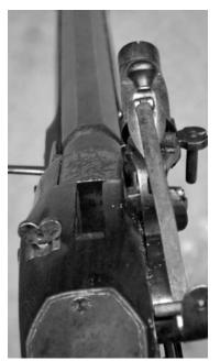
10. A firer's-eye view of the breech area of the rifle when preparing to fire. Note the offset peep-sight on the left.
