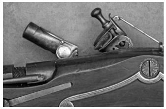
7. The nearside of the cock, showing the upper of two small holes in the throat, and of the priming magazine frizzle showing a small redundant screw. These would have allowed the fitting of a link bar.
