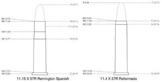
Figure 2. Dimensions of the .43 Spanish and Reformado cartridges.
