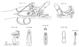
14. Sheet 3 of Thomson's patent illustrations (Figs. 17 to 23); an automatically-priming lock.
