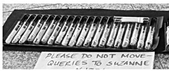
Figure 6: Textile samples left in bright light to assess photolytic degradation.
