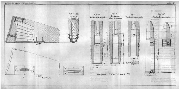
Figure 3. Original diagramme of proposed modification of .43 Spanish rifle to Reformado.
