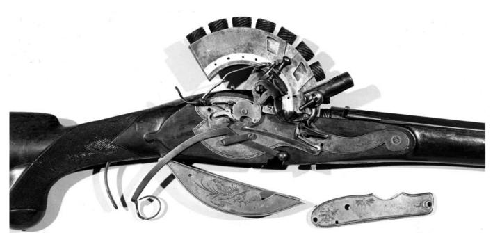
5. The lock mechanism with the cover plate removed.
