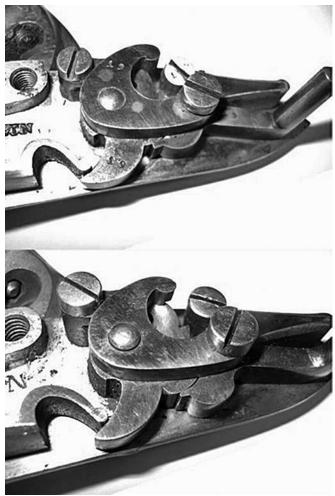
internal views of the same locks – the major difference is the lack of any assembly marks/numbers on le Blanc's lock (bottom)
