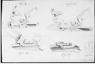
19. Original drawings for Thomson's designs for vertically sliding touchhole covers. Figs. 24 to 26 use a rocking bar, that in Fig. 27 is operated simply by the movement of the mainspring.
