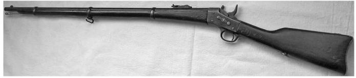
Figure 1. The well-worn 3rd contract Remington-manufactured No.1-model Rolling Block rifle (Remington model 71) in .43 Spanish calibre found to have disappointing accuracy. Replacement cleaning rod and rear sling swivel courtesy of Kenn Womack.
