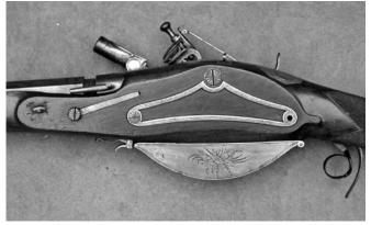
9. The sideflat showing the sham sideplate. Note on the left the spring catch for the breech piece.
