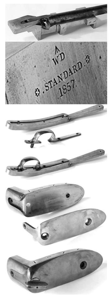
Figure 9. Gauges used in the manufacture of Enfield Pattern '53 rifles (all gauges are Royal Armouries, PR.10142).
