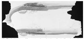
15. The bottom two of four watercolour sketches of a duelling pistol with its lock removed. They have additional rough sketches of Thomson's breech piece design.
