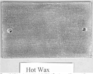
Figure 13: Mild steel coupon treated with hot Renaissance Micro-crystalline wax.
