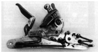
25. Interior of the Egg "Patent" musket, showing the rocking lever which moved the touch hole cover.
